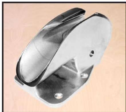
ANCHOR FAIRLEAD CN7609 Designed to use with windlasses. With nylon pulley, for up 9/16" Rope. For 1/4" - 5/16" Chain. 3-1/2" x 3-1/2". 316SS.
