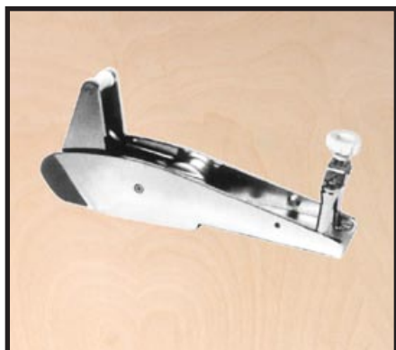
ANCHOR ROLLER for Bruce/Delta CN7614 Anchor Roller. 16" L x 3-3/8" W x 2-1/2" H. For Bruce/Delta Anchors. Max 12KG. Fits 1/4"-5/16" Chain.
