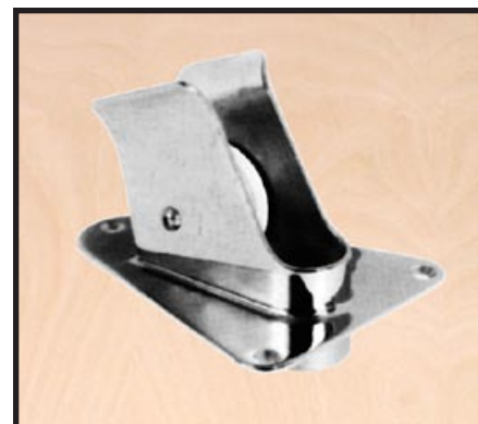
ANCHOR ROLLER for Inflatables CN7613 Designed to be fitted to fibreglass triangle at bow of inflatable. For up to 10Kg Anchor. Fits 1/4" Chain. 7-1/4" x 8-1/4". 316SS.
